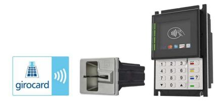
The cVEND PIN terminal for vending, parking and fueling machines was the first electronic payment device ever to receive electronic cash (girocard) type approval from the German Banking Industry Committee (DK) in accordance with the latest specification TA 7.2 / DC POS 3.0.
