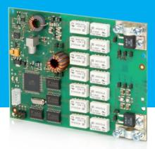
The Dynamic Antenna Tuner ID DAT is designed for automatic tuning and retuning of RFID Long Range Antennas with an operating frequency of 13.56 MHz. The parameters for setting the antenna are measured on the board under operating conditions. The antenna tuner is also able to disconnect the antenna circuit through an electronic switch up to a certain power.
