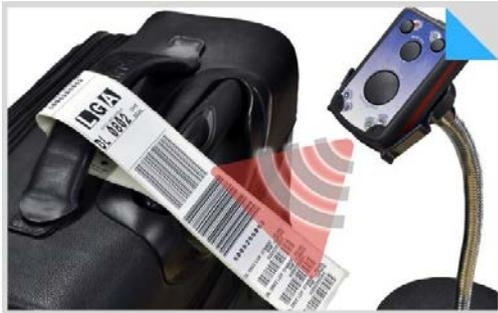
The mobile hybrid scanner "ECCO+" (RFID & Barcode) of FEIGs PANMOBIL product line first reads the barcode information printed on the barcode banderol and then writes this same information onto the IATA-conform RFID transponder that has also been attached to the banderol.
