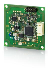
Designed with precision and versatility in mind, the ID CPR70 is a small RFID reader measuring just 5 cm x 5 cm. This cutting-edge module supports contactless smart cards and transponders compliant with ISO / IEC 14443 A / B, ISO 15693, and ISO 18000-3M3 standards. Its compact size and advanced features make it ideal for integration into terminals, printers, handheld devices, and various other applications.
